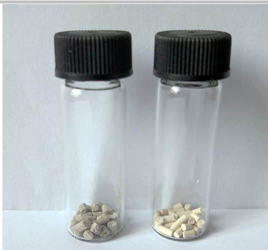
Figure S18. The photographs of molded Mg-gallate (left) and molded UOP zeolite 13X (right).
