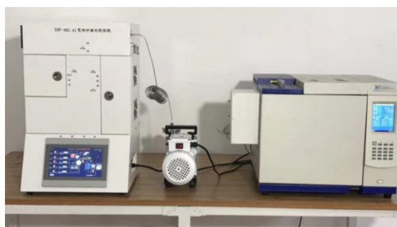
Figure S10. View of the automatic breakthrough equipment designed and used in our group.
