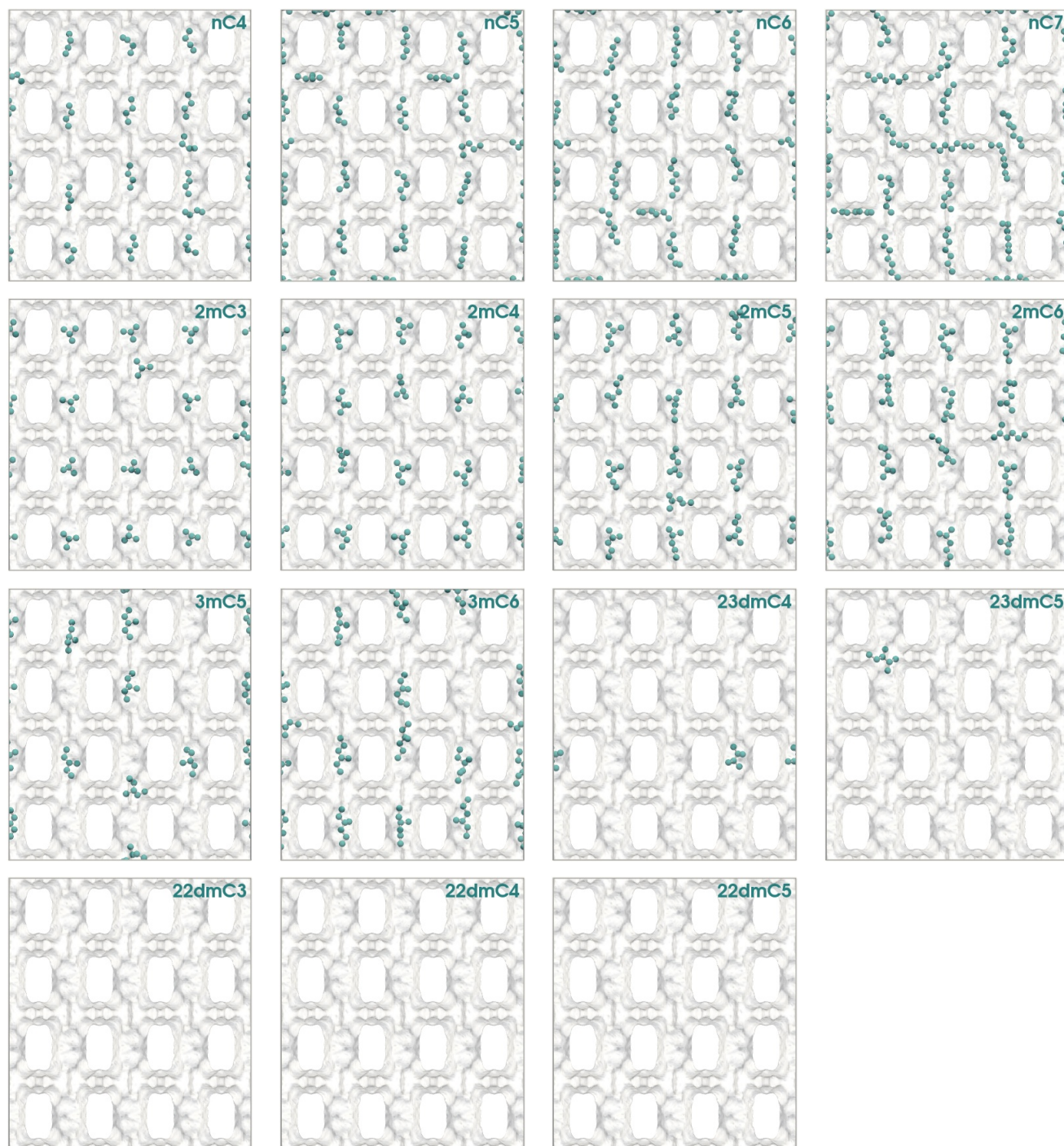
Figure S63: Simulation snapshots of (single-component) C4, C5, C6 and C7 isomers in ZIF-77 at 433K and 100 kPa. The structure is shown as a top-view of a single 2D layer of a 4 \times 2 \times 2 super cell. The main channels run top to bottom; the smaller side channels run from left to right and are only accessible to linear alkanes.
