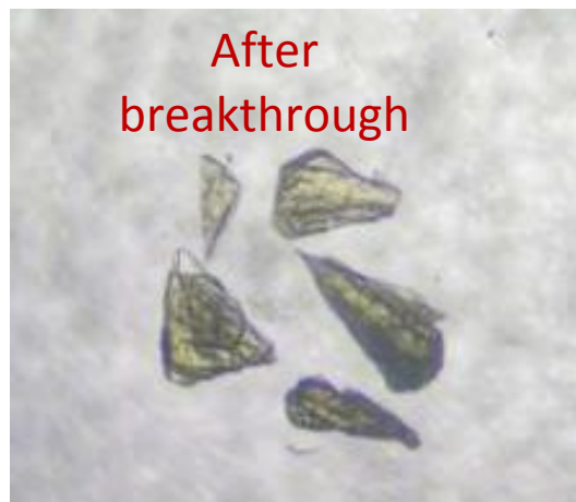
Figure S9. The photograph of ECUT-100 and the samples after breakthrough tests.
