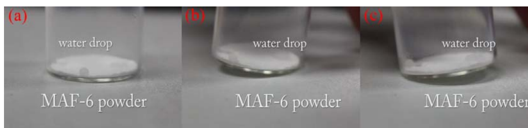
Figure S7. Snapshots of water droplet maintaining its shape (a) and rolling (b and c) on the powders of MAF-6. See supplementary movie for detail.
