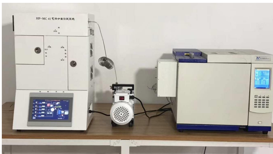
Figure S34. View of the automatic breakthrough equipment designed and used in our group.
