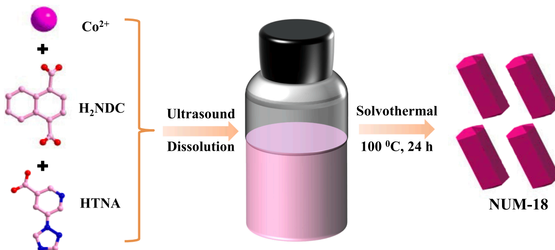
Fig. 1. Schematic illustration for self-assembly process of NUM-18.
