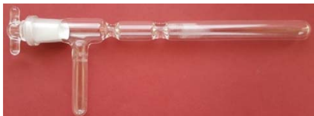
Fig. S1. Glass device for the hydrothermal healing procedure of the zeolite at 400 °C and 30 mbar water pressure.
