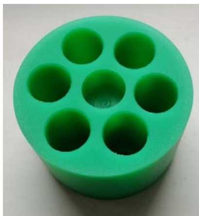
Fig. S4. Cooling device, which can be filled with liquid nitrogen. The glass tubes are placed into the inner hole. The outer holes are deeper and used for an additional cooling of the device.
