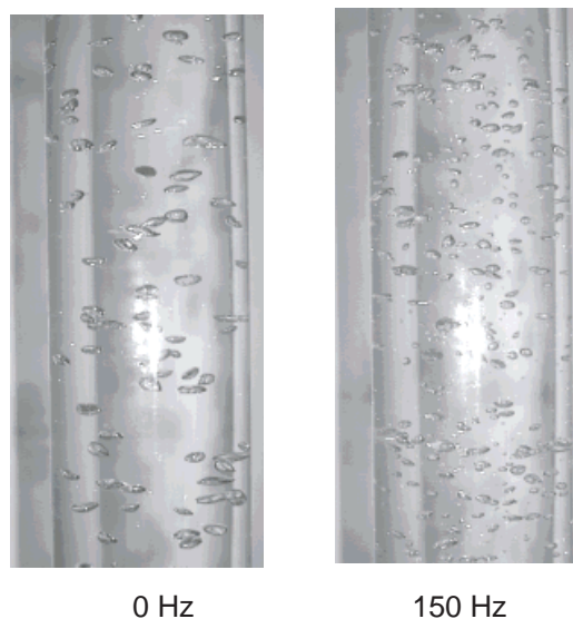
Figure 6. Photographs of bubble dispersion in air-water system with sieve plate distributor comparing no-vibration case with 150 Hz-vibration situation. Operation at superficial gas velocity U = 0.0011 \text{ m/s} .
