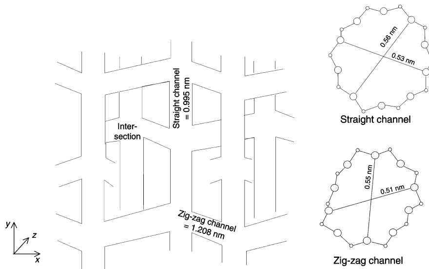
Fig. 3 Schematic of structure of MFI (silicalite-1). The cross-sections of the straight and zig-zag channels are shown in the inset.
