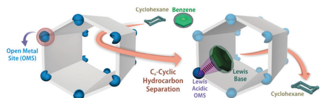
Scheme 1 Schematic representation of the pursued strategy: exploiting Lewis acidic coordinatively unsaturated sites of an OMS-rich MOF platform, to exhibit selective interplay with aromatic, planar Lewis base benzene over its aliphatic, non-planar C 6 -analogue cyclohexane.
