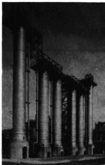
Figure 14. Photograph of the reactor section of a trickle-flow residue hydrodesulfurizer of 7000 t/day design capacity.
